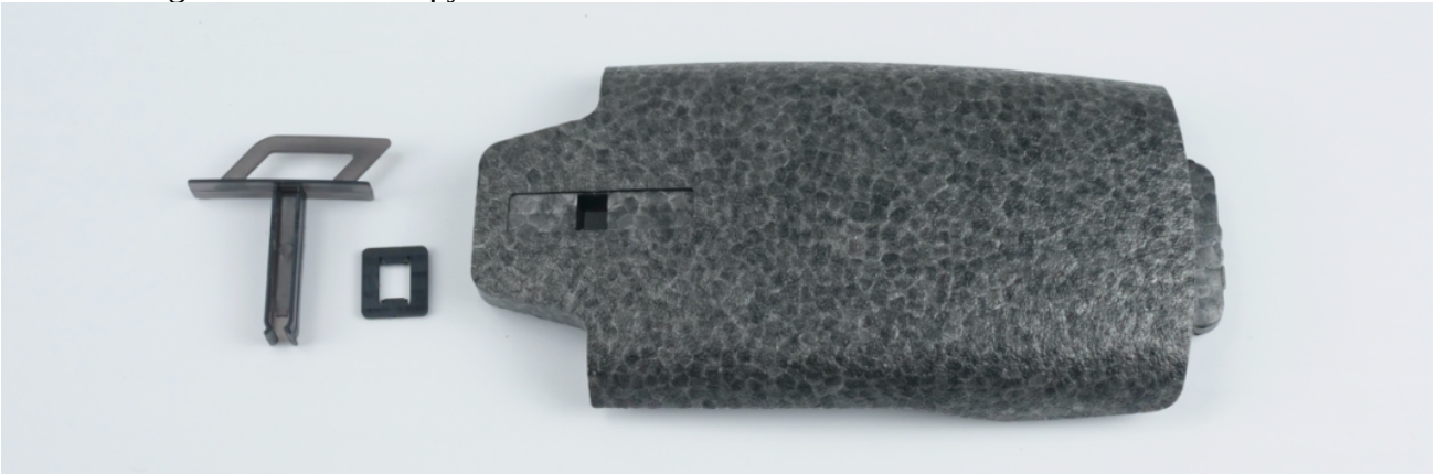
ab. Installing latch of the canopy
