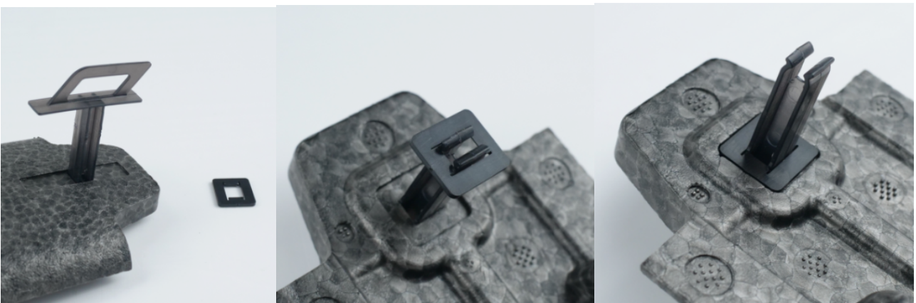
ac. Slot the latch through the canopy and secure it with the clip. The flat side of the clip facing outside.
